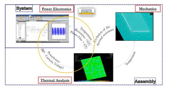
Power module cosimulation example – courtesy Safran
