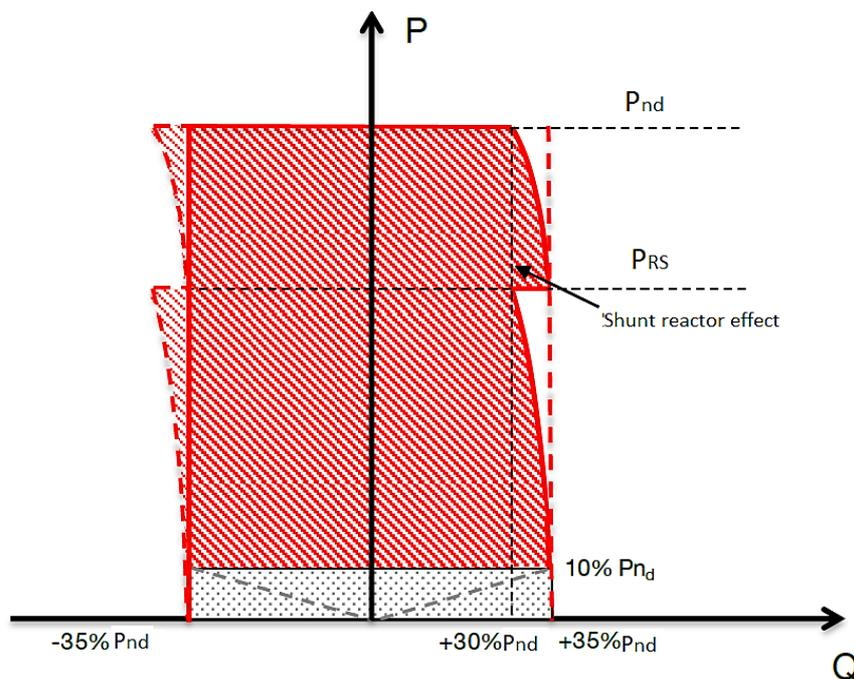
Figure 14: Requirements on reactive power provision capability for Type 2 wind plants [22].
