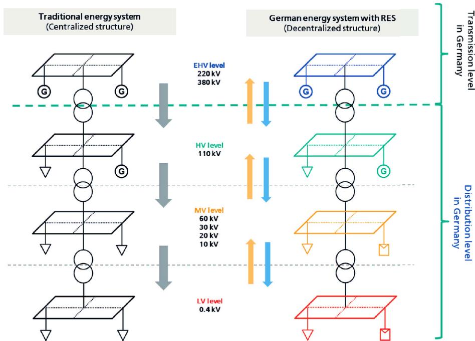
Figure 19: German energy system changes due to increased penetration of RES [2].
