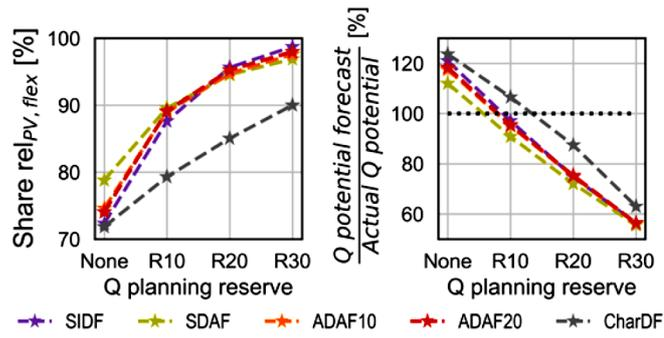
Figure 29: Share of reliable reactive potential forecast (left) and ratio of forecasted reactive power energy potential to actual reactive power energy potential (right) in daytime hours [30].
