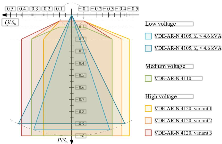
Figure 3: Requirements on reactive power provision capability for DER (based on [9–11])
