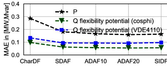
Figure 27: Mean absolute error of PV forecasting methods in daytime hours [27].
