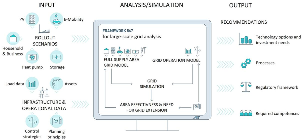
Figure 35: Methodology for large scale power system analysis.
