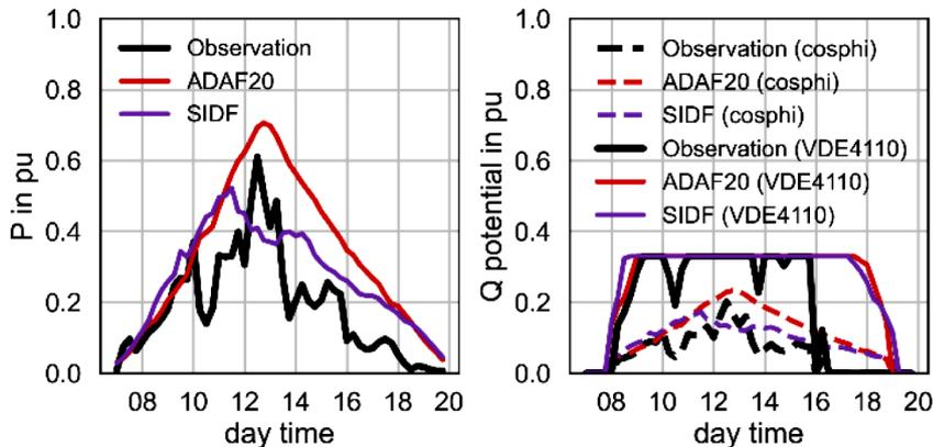
Figure 26: PV active power feed-in (left) and reactive power flexibility potential (right, overexcited) [27].
