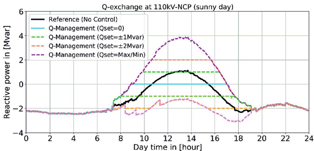
Figure 33: Reactive power exchanges at 110 kV-NCP with different reactive power setpoints [8].
