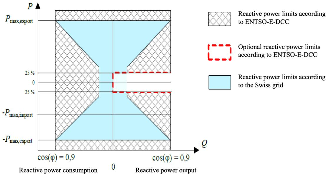
Figure 17: Reactive power limits of loads and distribution systems with the transmission system according to ENTSO-E-DCC [25] and to a Swiss regulation [26].
