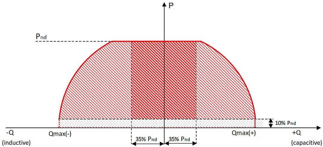
Figure 12: Requirements on reactive power provision capability for Type 2 PV plants [21].
