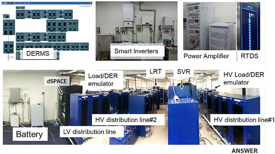
Figure 37: Overall of the hardware testbed.
