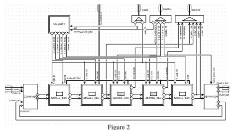
Model structure of the circulation tanks
